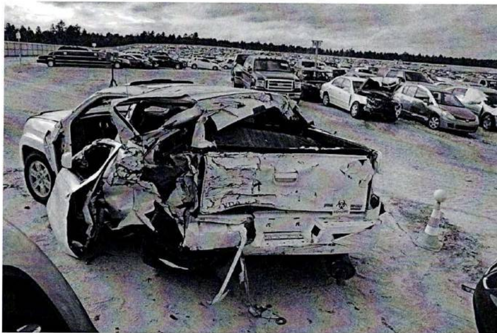
Figure 6. Rear damage to Honda Ridgeline
