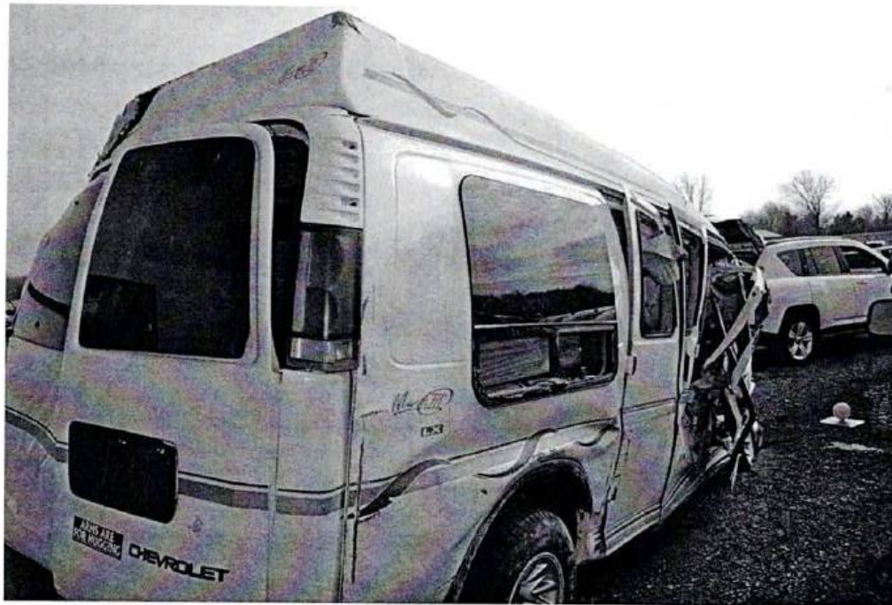
Figure 5. Rollover damage to passenger's side of Chevrolet Van
