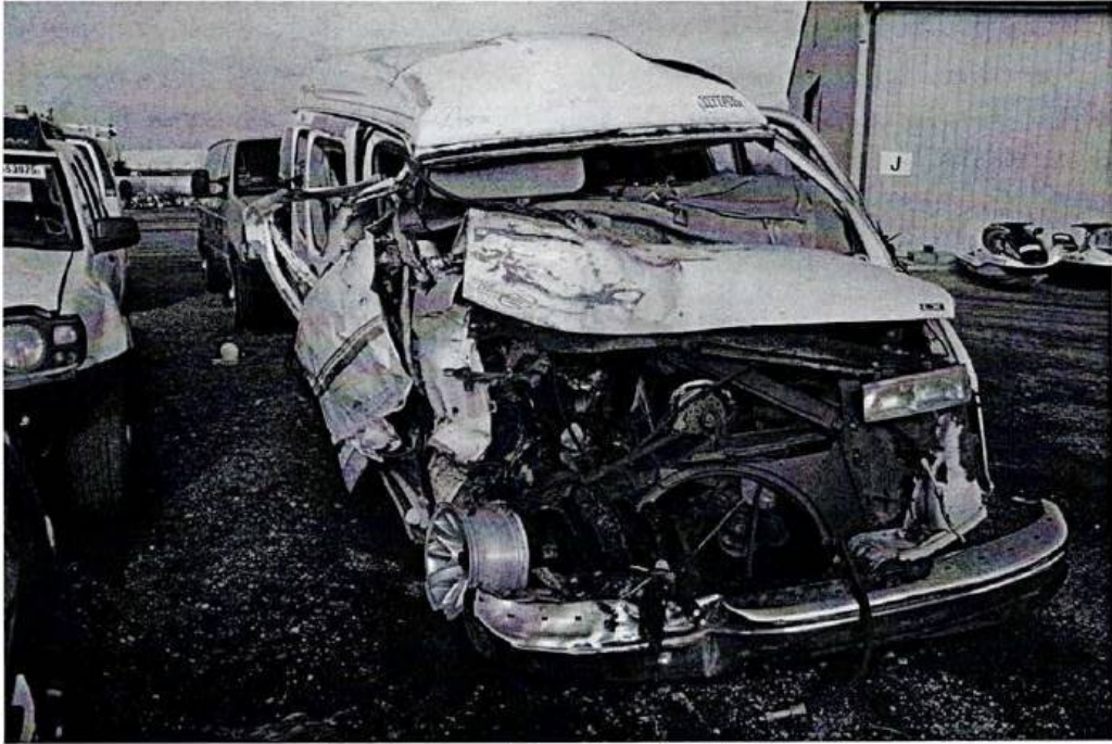
Figure 1. Frontal damage to Chevrolet Van
