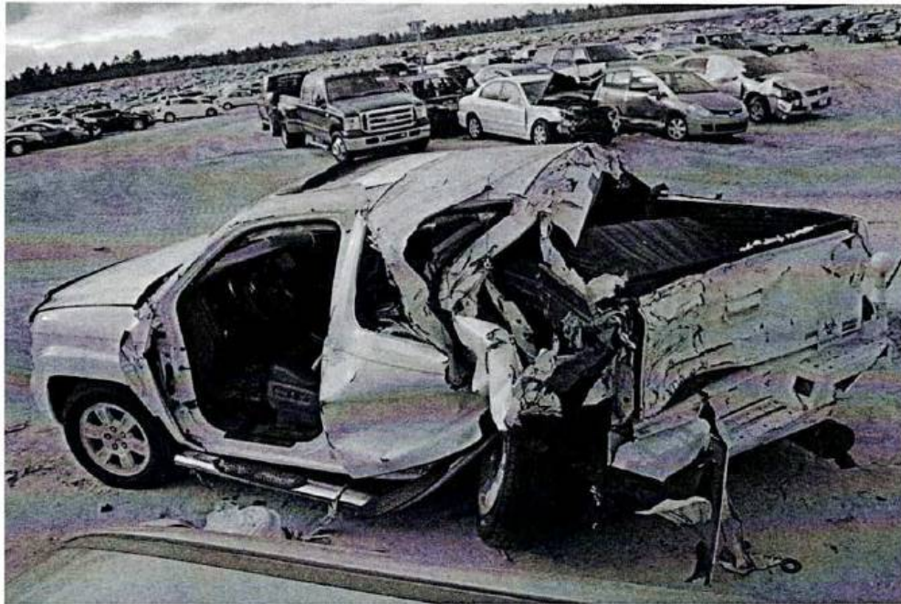
Figure 7. Driver's side rear damage to Honda Ridgeline
