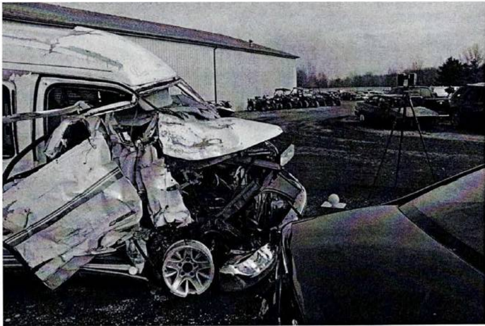
Figure 3. Frontal damage to Chevrolet Van
