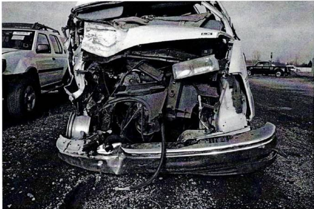
Figure 2. Frontal damage to Chevrolet Van
