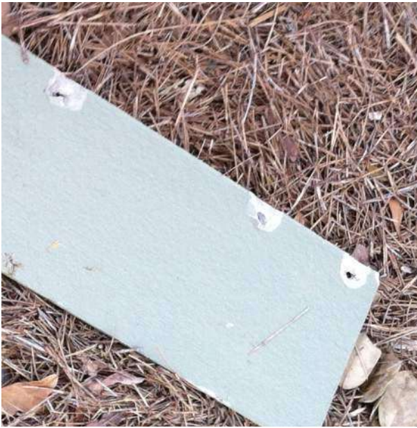
Countersunk Nail Holes With No Second Nail and Wrong Spacing
