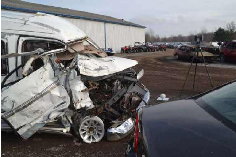
Figure 3. Frontal damage to Chevrolet Van
