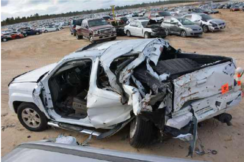
Figure 7. Driver's side rear damage to Honda Ridgeline
