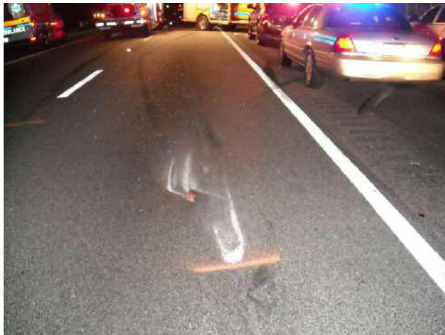
Figure 2. Collision related marks in the impact area
