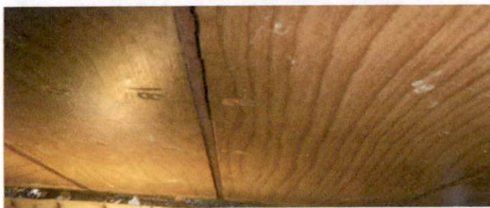
Fan blades warped from excessive humidity.
