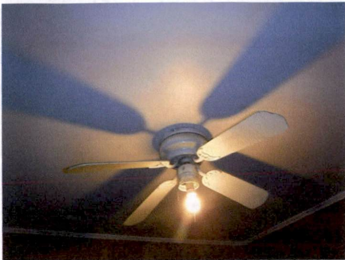
Fan blades warped from excessive humidity.
