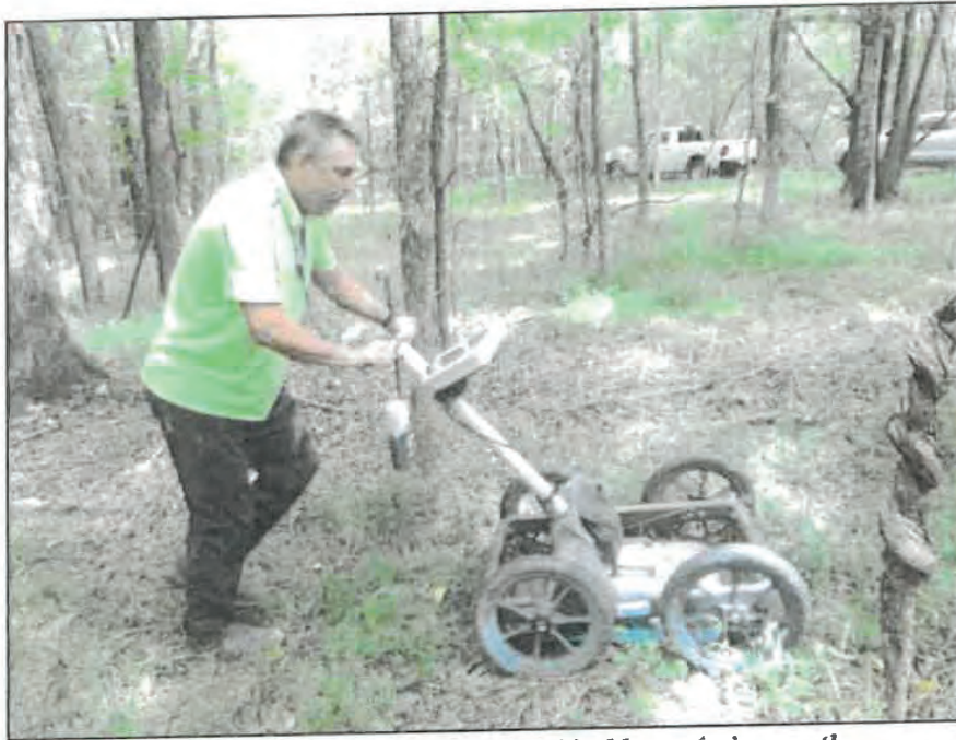
Figure 16. GPR portion of geophysical survey of area behind barn, facing north.
