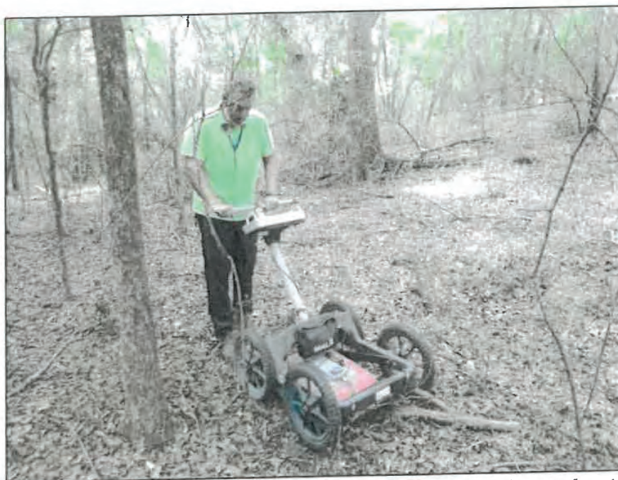
Figure 18. GPR portion of geophysical survey of area near spring head, facing southeast.
