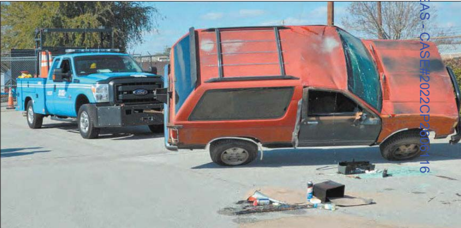
John Weaver of Parsons Corporation shows SCDOT Incident Responders the best place to attach a chain to turn over a flipped vehicle.
