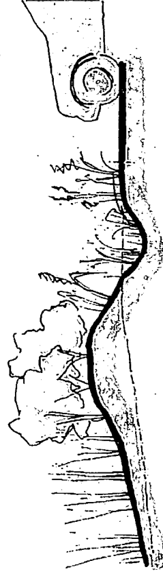
Vegetated bioswales capture and treat stormwater runoff from parking lots
